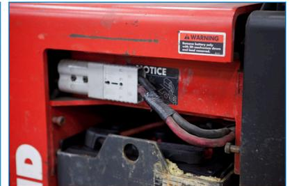
*Inspect cables for damage*
