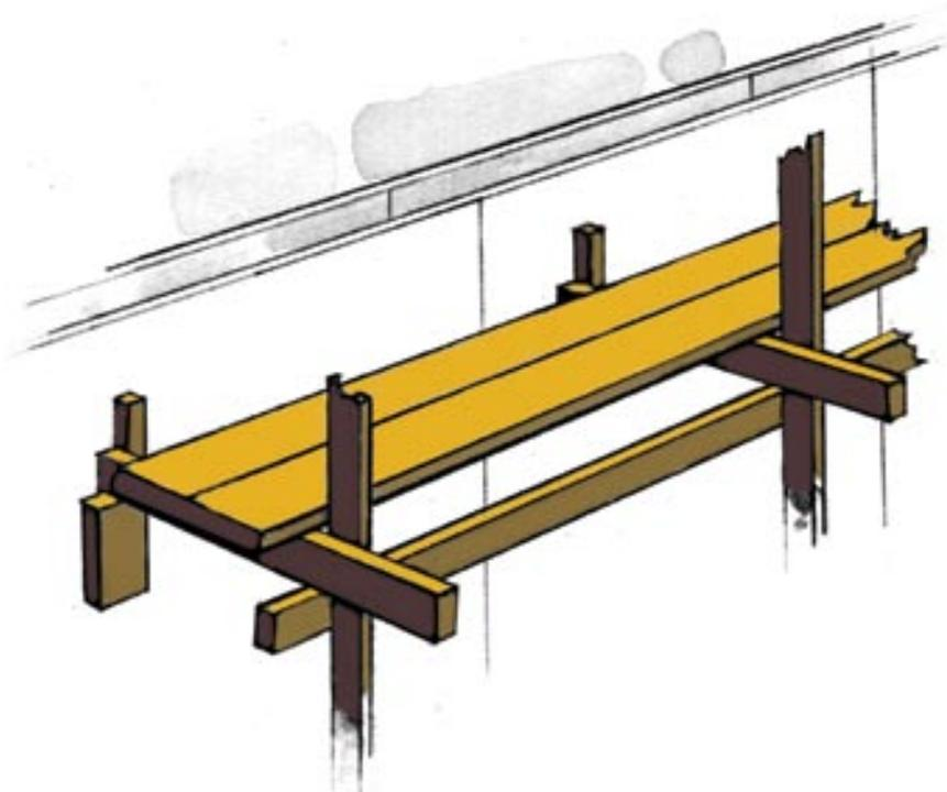
*Single-pole wooden scaffolding for pouring or pumping concrete.*
