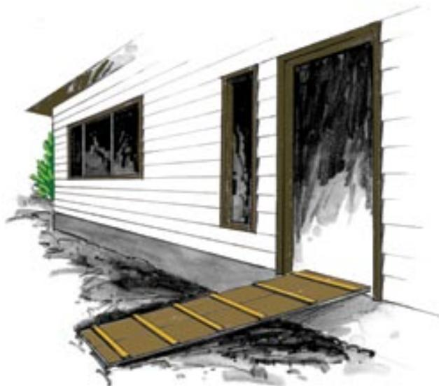
*The slope of work platforms must not exceed one vertical to five horizontal. Slope work platforms must have cleats spaced no more than 400 mm (16 in.) apart or a non-skid surface.*
