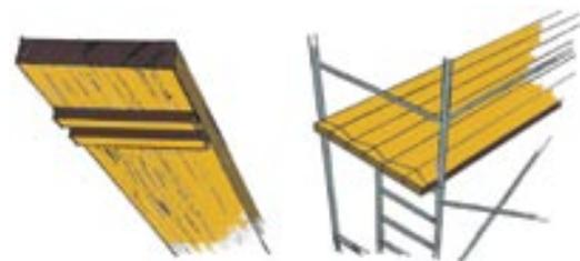
*Scaffold planks must be held in place if there is a danger of the planks slipping off their supports.*
