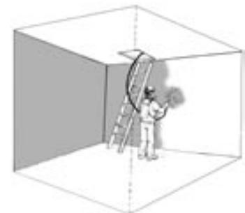
*This water cistern is a confined space with limited access and ventilation. While a waterproof coating was being applied, flammable vapours were generated. The vapours ignited, and an explosion occurred. One worker died, and another was severely injured.*
